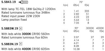
With leds white 4000K CRI90 605Im Rated luminaire luminous flux 66lm
