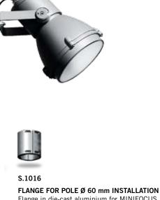
Flange in die-cast aluminium for MINIFOCUS, suitable only for Ø 60mm poles. To install the flange on Ø 76mm pole the screws kit SACVITFOCTOWER2 must be purchased separately. The flange can be used for maximum 2 projectors, one for each side.
